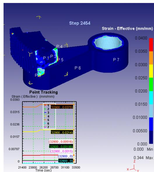
Fig. 4. Plastic deformation in the wheel segment.
