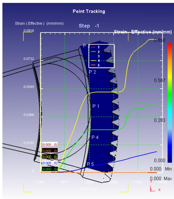
Fig. 5. Effective (plastic) strain in the existing heating schedule.
