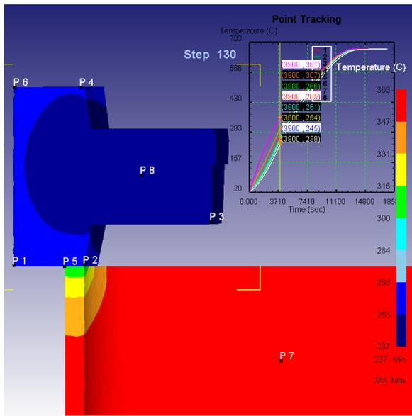
Fig. 1. Maximum temperature difference between the base and the work.
