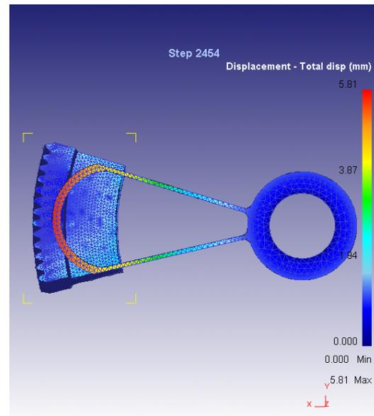
Fig. 2. Expansion of the base under the wheel at the end of the heating process.
