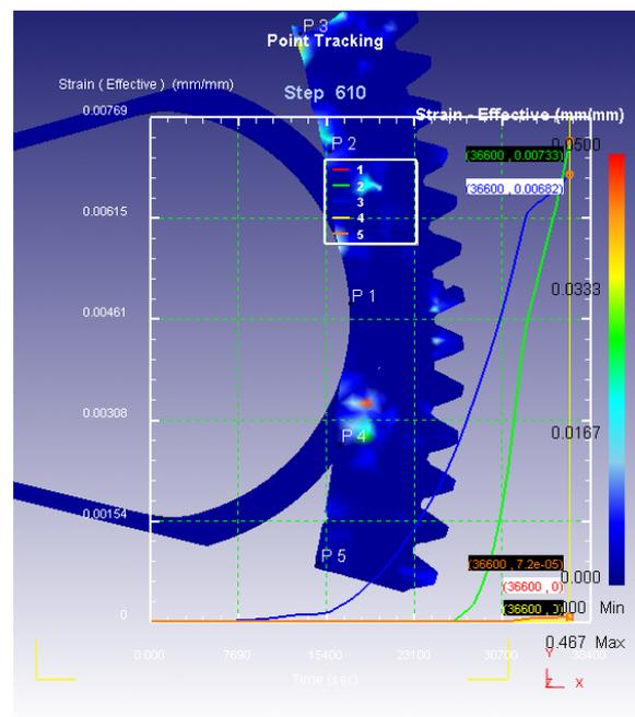
Fig. 6. Effective (plastic) strain in the heating schedule 2.
