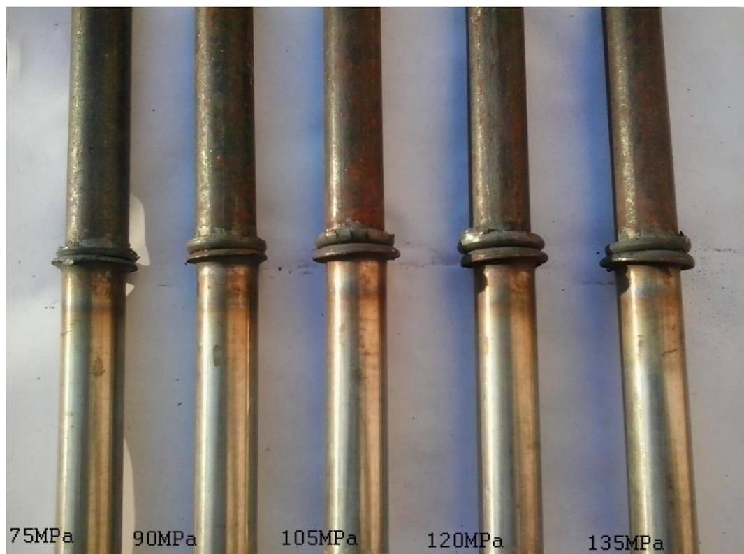
Fig. 1. Macrograph of the friction welded specimens at different axial pressures.
