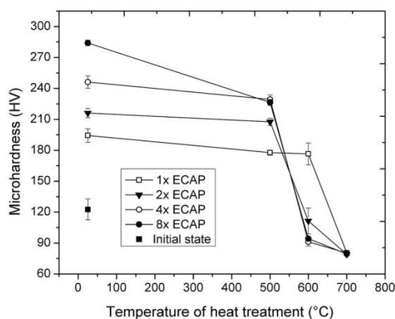
Fig. 3. Dependence of Vickers hardness on the temperature of annealing
