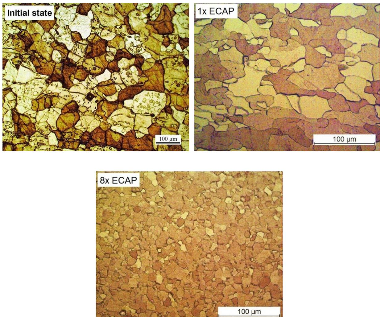
Fig. 4. Optical micrographs of initial state and samples annealed for 1 hour at 700 °C taken from the cross section
