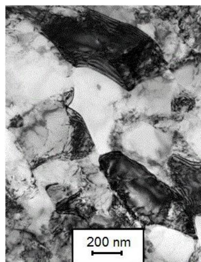
Fig. 2. TEM micrograph of the cross section of 8x ECAPed sample
