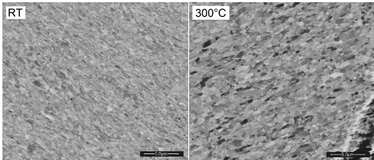
Fig. 7. SEM micrographs of the longitudinal section of 8x ECAPed sample deformed at room temperature and at 300 °C
