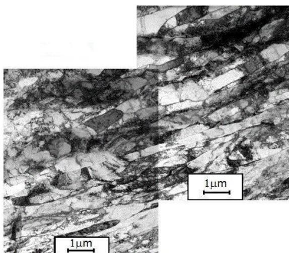
Fig. 1. TEM micrograph of the cross section of 1x ECAPed sample
