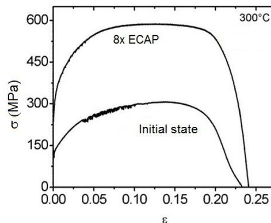
Fig. 6. Comparison of true stress-true plastic strain of initial state and 8x ECAPed samples, respectively, at 300 °C
