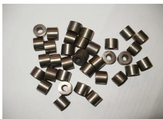
Fig. 2. Test specimens of pump material
