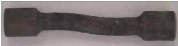
Fig. 3. Testing samples distortions (565 °C/32 hours)
