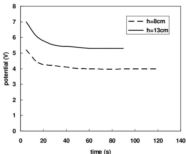
Fig. 7. Dependence of potential at constant current of 1A on time and distance ( $h$ ) between the electric contact and electrolyte level
