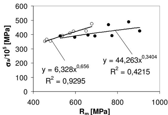
Fig.2 Dependence of fatigue strength on tensile strength of steels (full symbols – samples with  $t_{\text{coiling}} = 20$  °C)
