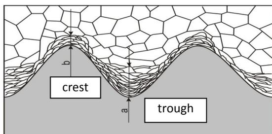
Fig. 3. Schema of evaluated thickness of deformed areas in Ti matrix
