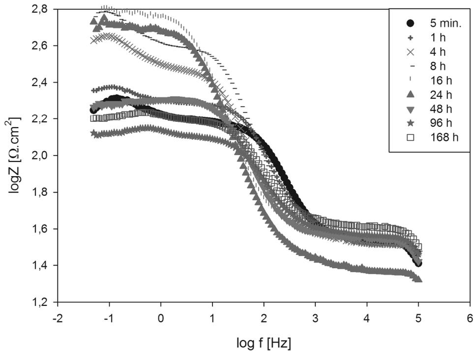
Fig. .3 Bode plots of the grinded surface of the AE21 Mg alloy in 0.1M NaCl after various exposure times
