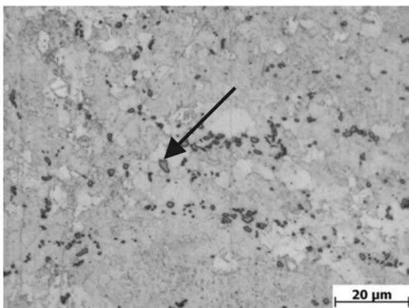
*Fig. 2.  $\text{Al}_4\text{RE}$  ( $\text{Al}_4\text{RE}$ ) phase detail, etch. picric acid [8]*
