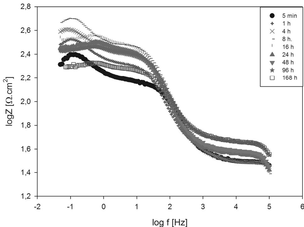
Fig. 4. Bode plots of the grinded surface of the AE21 Mg alloy in 0.1M NaCl after various exposure times
