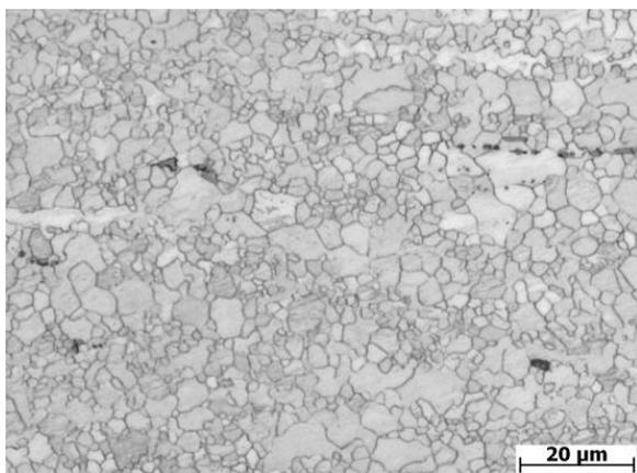
*Fig. 1. Microstructure of the AE21 EX magnesium alloy, etch. picric acid [8]*
