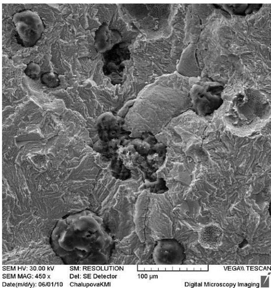
Fig. 7. Detail of fracture at  $K_a = 14 \text{ MPa.m}^{1/2}$
