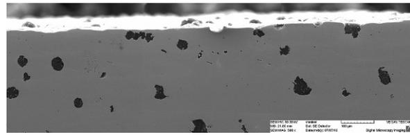
Fig. 4. Detail of fracture profile at  $K_a = 4 \text{ MPa.m}^{1/2}$
