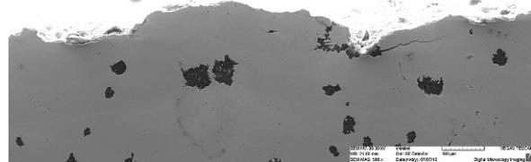
Fig. 5. Detail of fracture profile at  $K_a = 14 \text{ MPa.m}^{1/2}$
