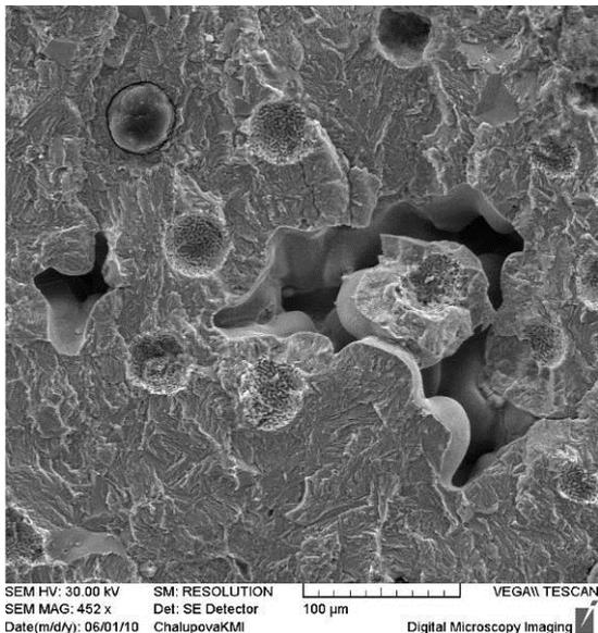
Fig. 6. Detail of fracture at  $K_a = 4 \text{ MPa.m}^{1/2}$
