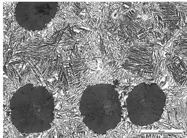
Fig. 1. The microstructure of ADI 1050, etched with 3 % Nital
