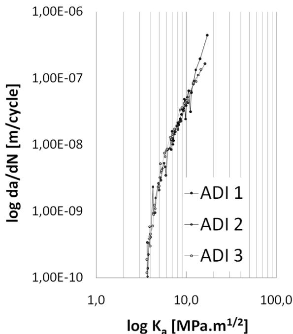
Fig. 3. Fatigue crack growth rate data of ADI 1050
