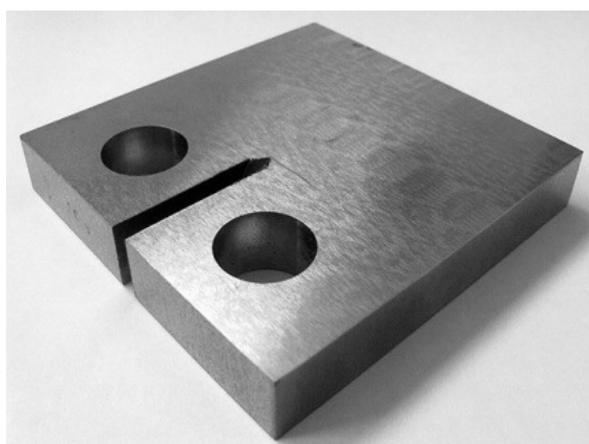
Fig. 2. Compact tension specimen
