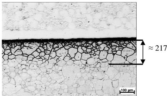
Fig. 9. The width of NI 102 (02) brazing alloy's diffusion into AISI 321 (1050 °C / 30 min.) [μm]
