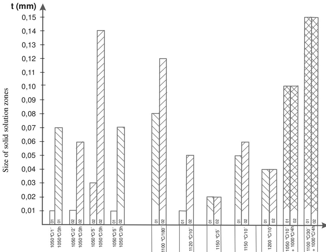
Fig. 7. The size of solid solution zones (t) for NI 102 (01) and NI 102 (02) brazing alloys in dependence on brazing conditions
