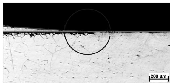
Fig. 5. NI 102 (02),  $\alpha \sim 5.14^\circ$  (1050 °C/ 30 min.)
