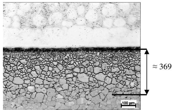
Fig. 10. The width of NI 102 (02) brazing alloy's diffusion into AISI 321 (1050 °C / 120 min.) [μm]
