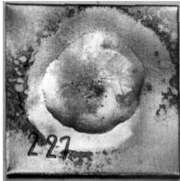
Fig. 1. Sample of fluidity of highly alloyed austenitic steel with Ni brazing alloy
