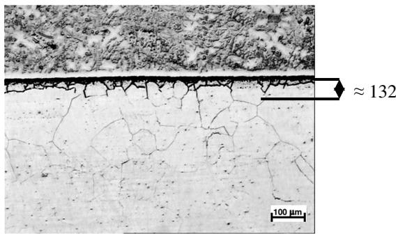
Fig. 8. The width of NI 102 (02) brazing alloy's diffusion into AISI 321 (1200 °C / 10 min.) [μm]
