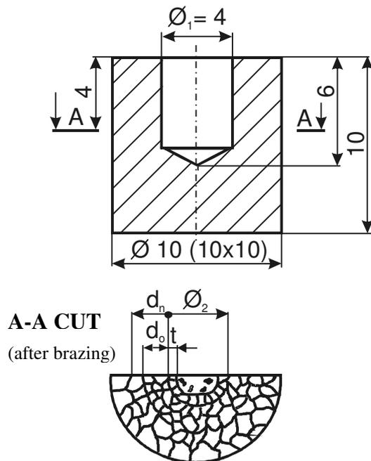
Fig. 2. Sample taken for the purposes of ascertaining the degree of BM's dissolubility (erosion) in Ni brazing alloy
