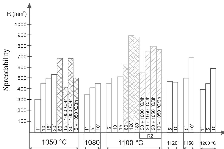
Fig. 3. The results regarding the NI 102 (01) brazing alloy's spreadability  $R$  ( $mm^2$ ) in dependence on brazing conditions
