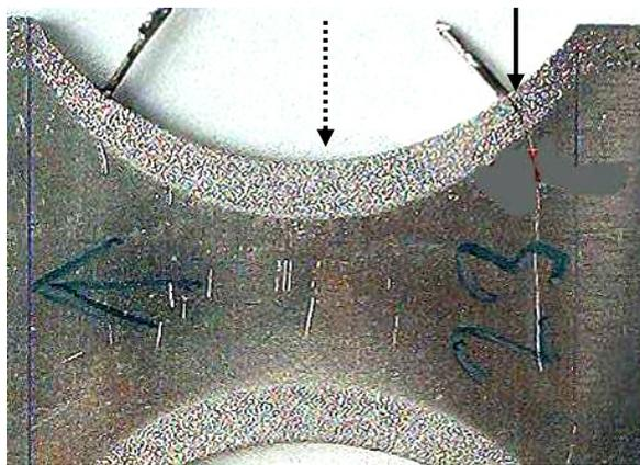
Fig. 10. Crack initiation under electrode (upper right) in shot peened specimen with 0.35 mm preliminary crack
