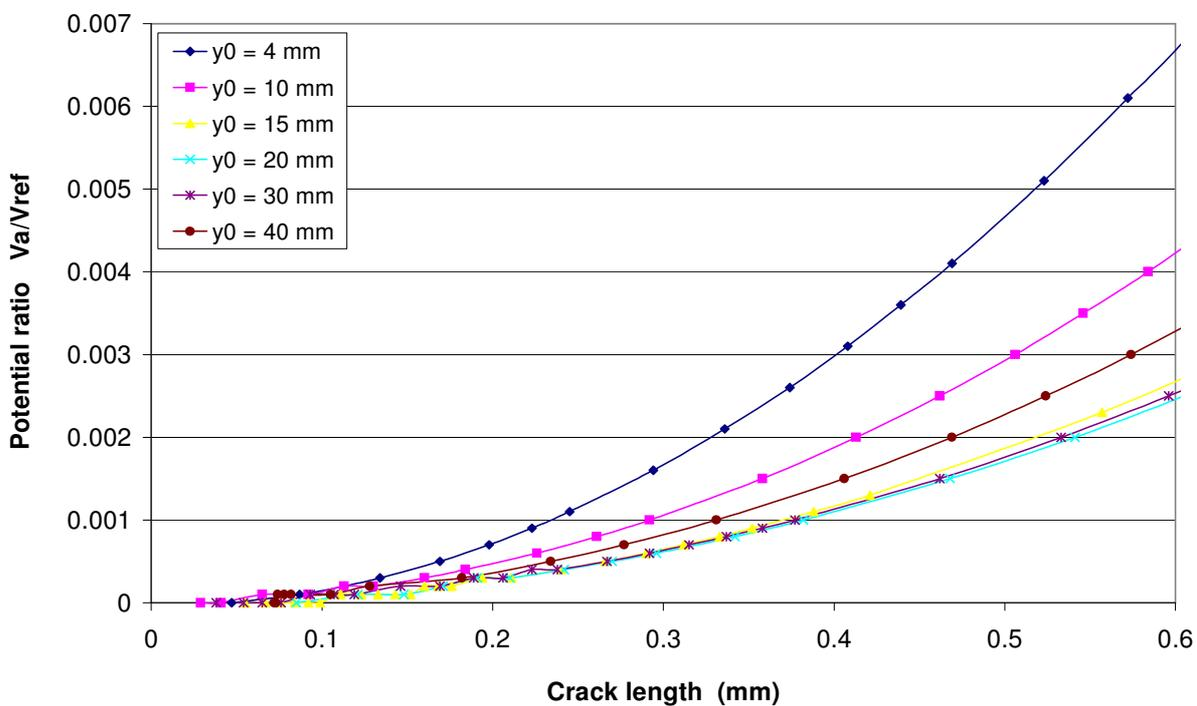
Fig. 2. Detailed DCPD sensitivity analysis on distance of electrodes for very short crack lengths
