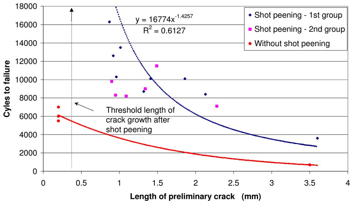
Fig. 9. Fatigue life after application of shot peening in comparison with untreated specimens
