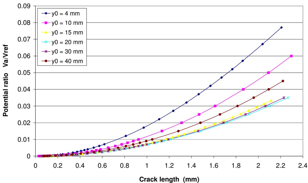
Fig. 1. Analysis of DCPD sensitivity on distance of potential electrodes from crack mouth
