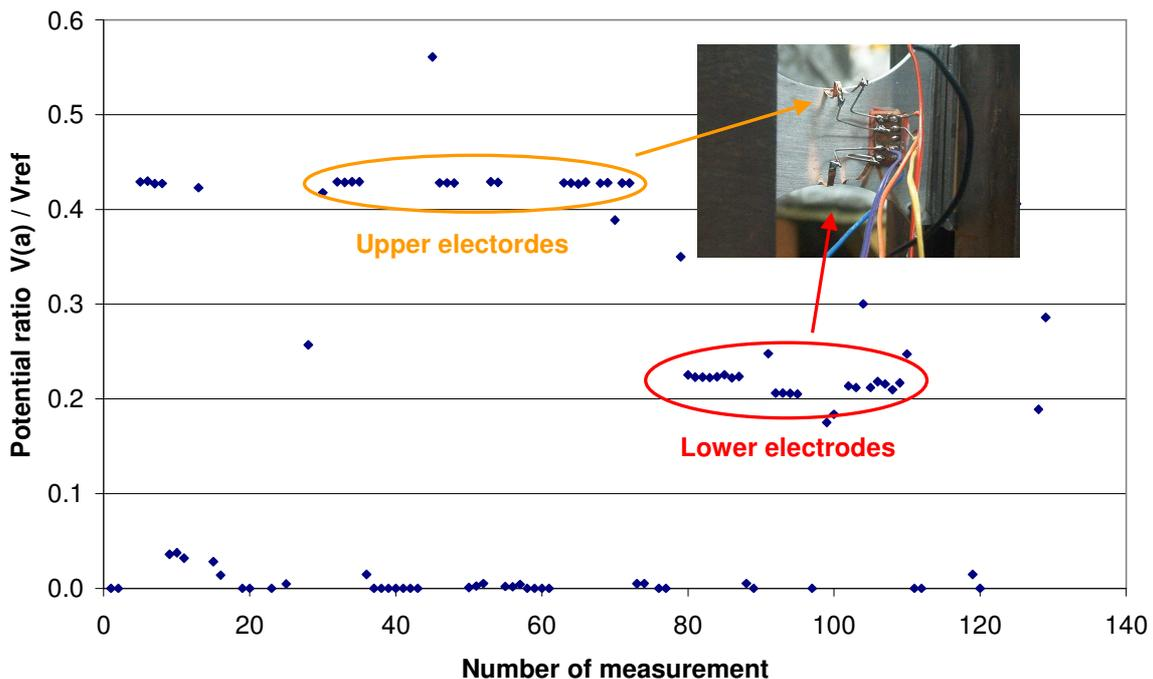
Fig. 4. Verification of use of self-adhesive Cu strips as potential measurement electrodes
