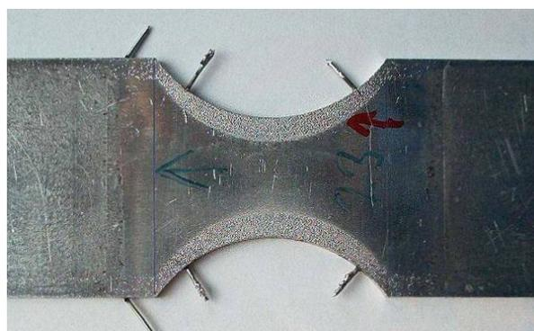
Fig. 8. Specimen after application of shot peening with potential and reference electrodes
