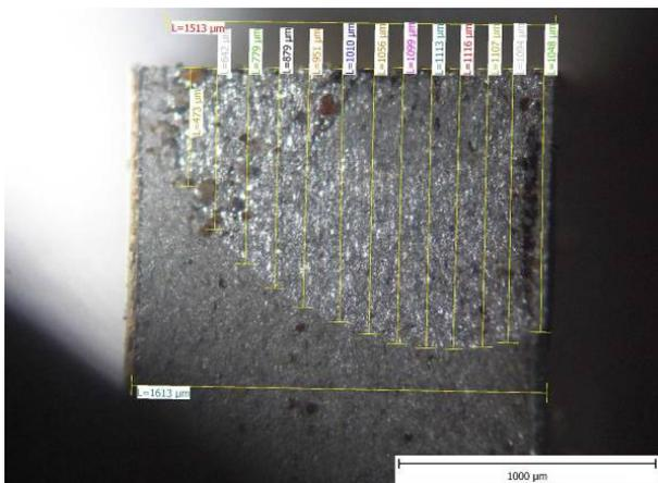
Fig. 6. Typical quarter-circular shape of short crack front initiated near the edge (upper right corner)
