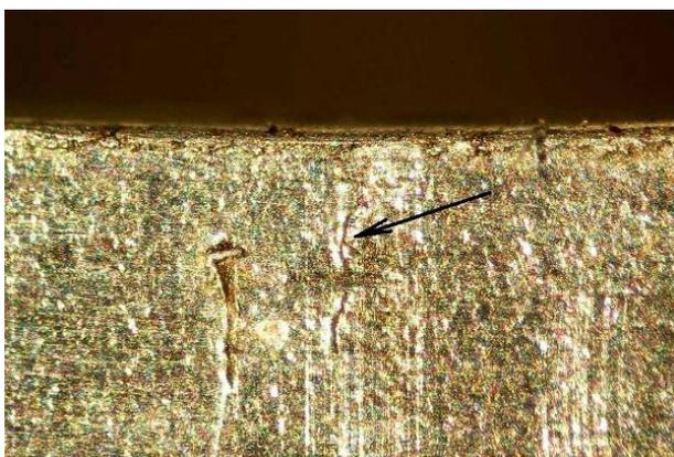
Fig. 7. Crack of surface length 1.05 mm, not visible in the area of specimen side – initiation site
