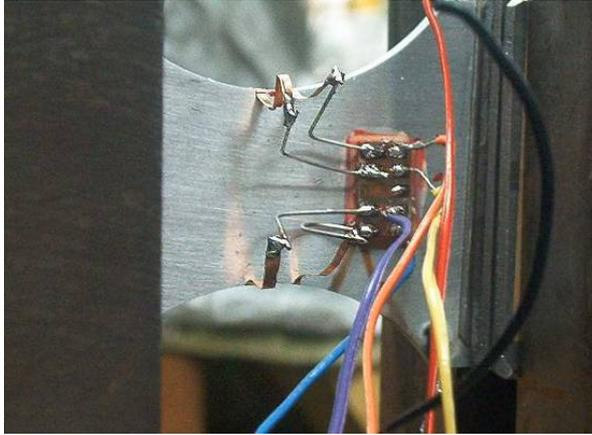
Fig. 3. Specimen with narrow Cu self-adhesive strips used as potential electrodes
