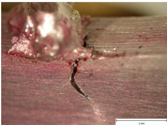
Fig. 5. Example of crack initiation under soldered potential electrode
