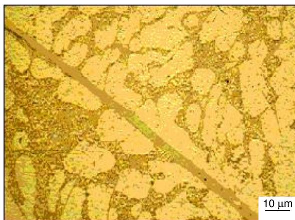
Fig. 1. The needle of β phase – FeSiAl<sub>5</sub>
