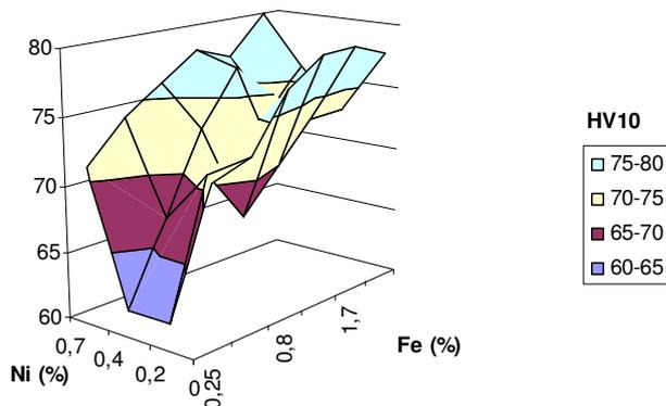
Fig. 5. The influence of Ni and Fe content on HV10
